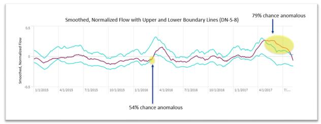
Figure 1: Example Dearborn meter DN-S-8 showing elevated flows due to river inflow in 2017, AI model detected the issue roughly three weeks after it began, and much before it was flagged in manual review
