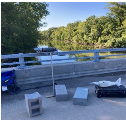
Water quality monitoring equipment set up by USGS on the Clinton River during a 2025 Watershed Hub Field Day event.
