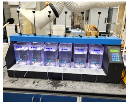
Jar testing at Water Works Park
