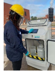
Figure 3: Chemist Niyla Reid operating the WAVE vacuum sampler at the Main Plant Influent 2 location.
