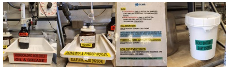
Figure 1: Baby Creek CSO basin sample preservation (left), guidance documents (middle) and new storage for fecal coliform sample bottles (right).
