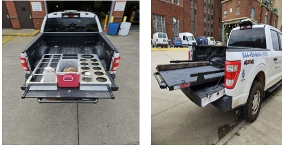
The truck bed slide-out with the fabricated sample holders installed on a laboratory truck
