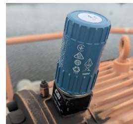
Wireless snap-on Vibration Transmitter used during site Survey
