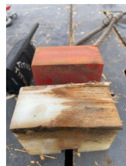
The new shoe material (red) next to the old shoe material (white). These shoes were installed new at the same time
