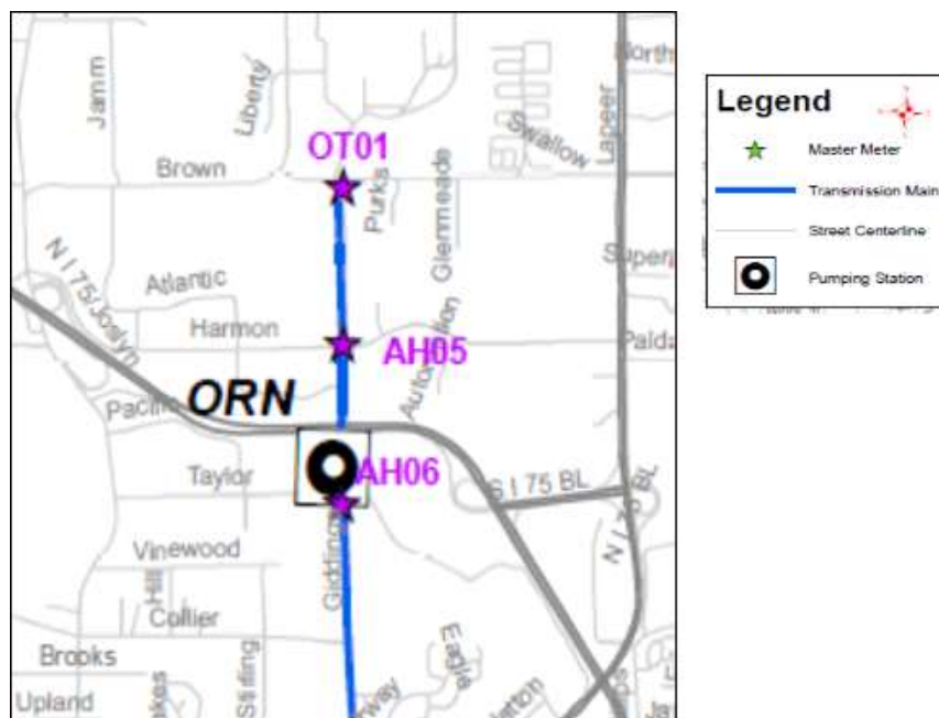
Figure 1: Orion Pumping Station Service Map
