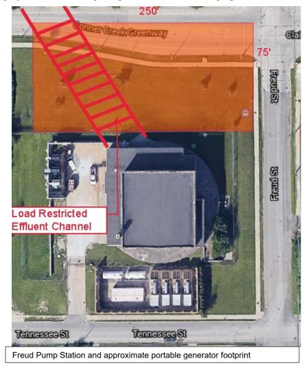
The orange box demonstratively shows the required footprint for portable generators relative to the facility. The red hatching is the effluent channel from Freud Pump Station to the Conner Creek Combine Sewer Overflow (CSO) facility. Since the effluent channel is shallow; an engineering review would be necessary to determine the loading capacity on top of the channel.
