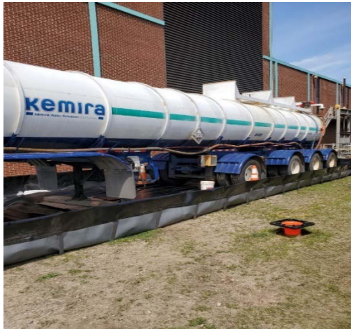
Temporary Chemical Tanker with Spill Containment
