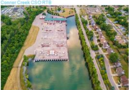
Figure 40. Conner Creek CSO RTB Detroit's largest CSO control facility, the Conner Creek CSO RTB eliminated three outfalls and has dramatically improved water quality in Conner Creek and the Detroit River since going into operation in November 2005. This RTB provides 62 million gallons of total storage, with 30 million gallons in the retention treatment basin and 32 million gallons in upstream structures. High-speed mixers are used to rapidly disinfect flows and achieve the required fecal coliform limits. This facility was sized to provide five minutes of detention for settling and disinfection for the peak flow from the 10-year, one-hour storm.
