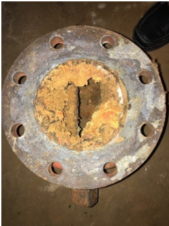
The photo shows the condition of the heating system hot water piping.
