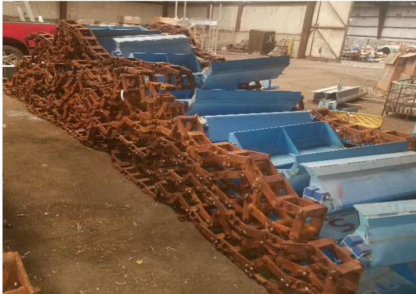
Replacement grit channel chain and buckets
