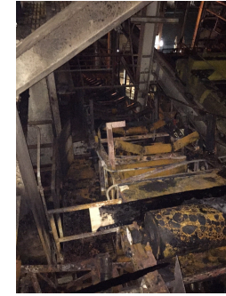
Picture from left to right Sludge Conveyor G Damaged by Fire and Conveyor B in the Complex – II Dewatering Building and Fire Damaged Conveyor H in Complex-II Incinerators Building
