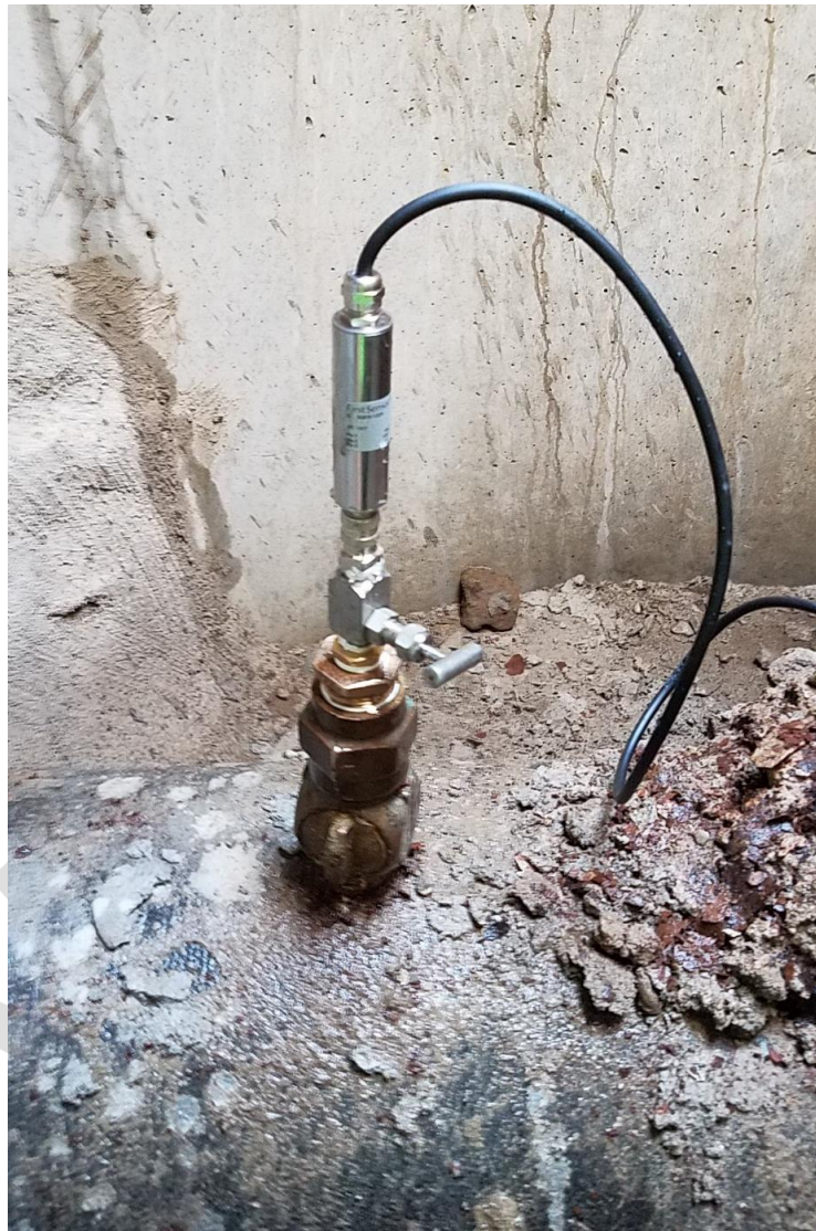
Figure 2-22 Example Installation of Pressure Logging Infrastructure
