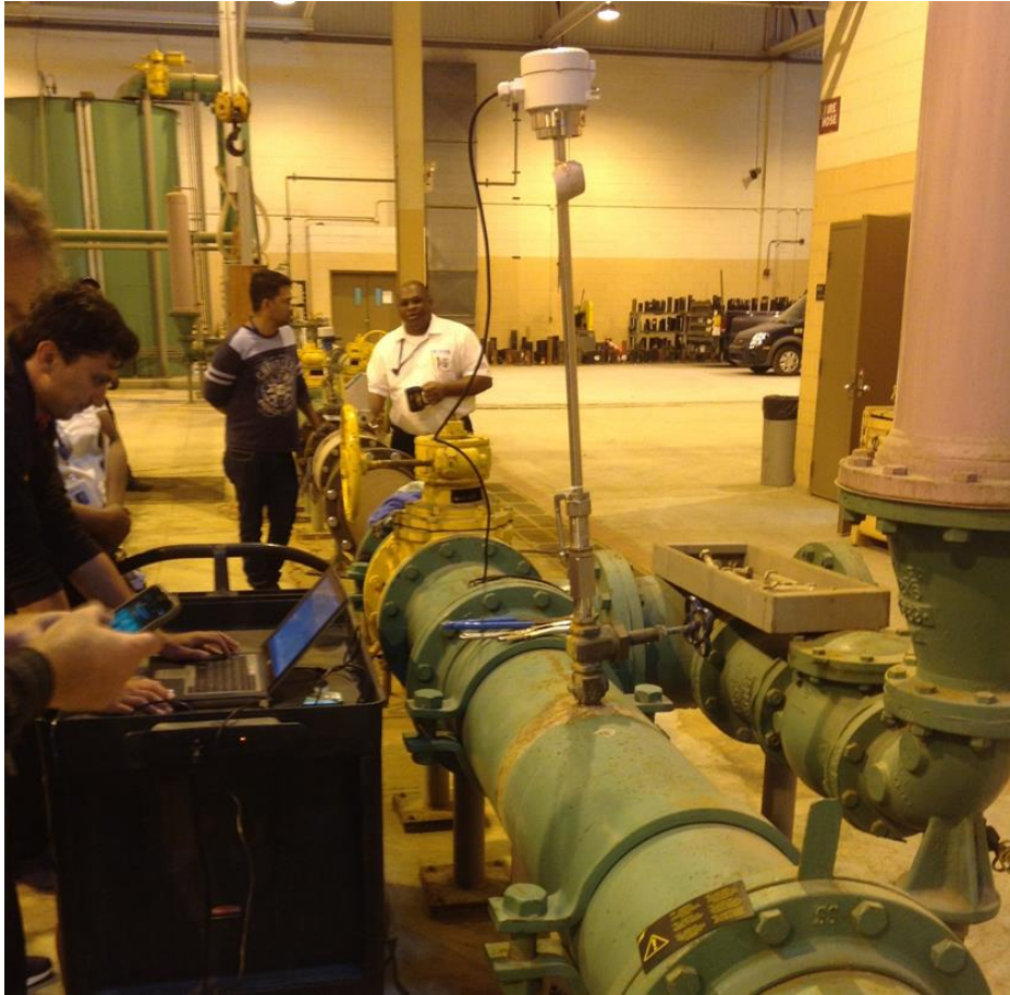
Figure 2-20 Insertion Flow Meter Test Bench Configuration
