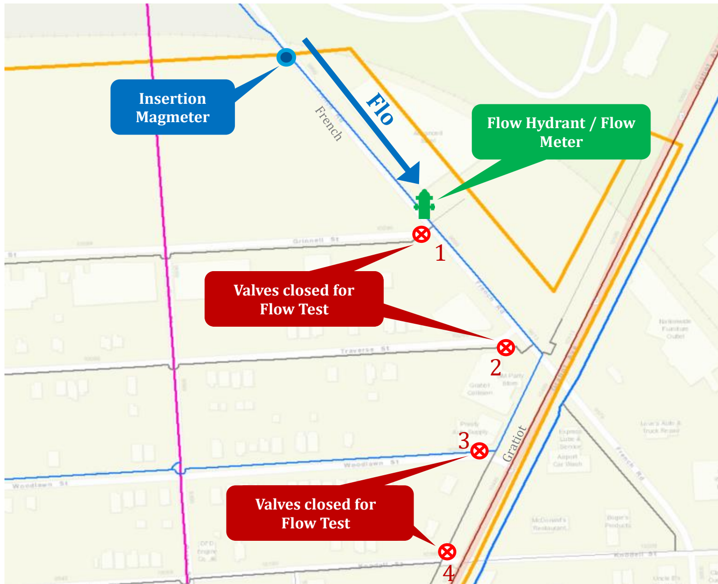
Figure 10-11 In-Situ Flow Test on French Rd. Meter
