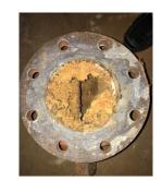
The photo shows the condition of the heating system hot water piping buildup which necessitates the complete replacement of the hot water radiant system in the filter building and other areas of the LH WTP.
