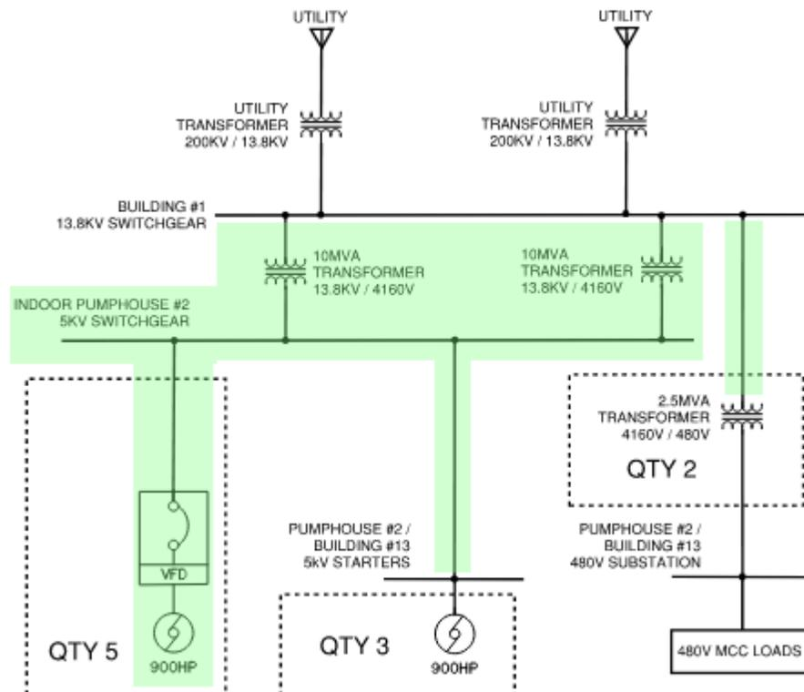
The only original medium voltage equipment kept in service would be the two 2.5MVA 13.8kV/480V transformers T-17 and T-18 within the 480V Unit Substation in Electrical Building #13. T-17 and T-18 power 480V MCC-P2-1 and MCC-P2-2 located in Electrical Building #13 and 480V MCC-P2-3 and MCC-P2-4 located in the Chemical Building. These two transformers would be repowered with 13.8kV from Electrical Building #1 which will require an outage on each.
