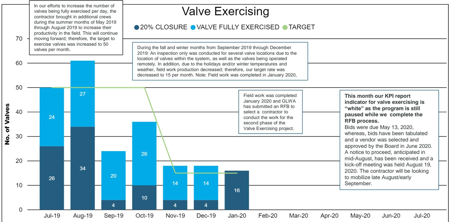
**Infrastructure Strategy and Performance:** GLWA's goal is to determine the status of system valves and prioritize necessary repairs. 450 valves will be evaluated and will be operated from open position to close and back open two times at a minimum.
