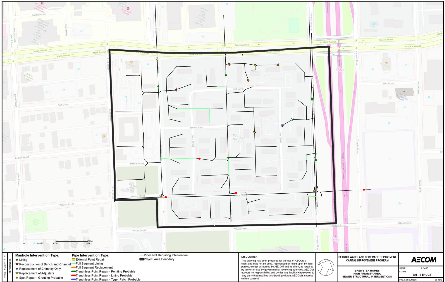
Figure 12 – Brewster Homes Sewer Structural Repairs
