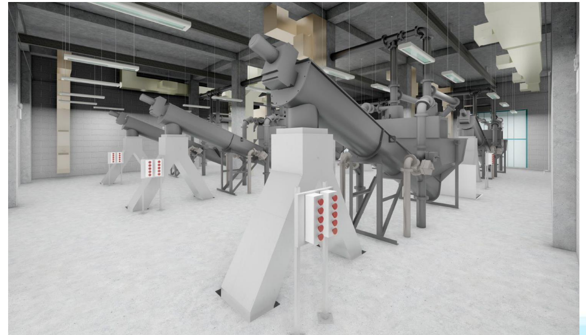
Grit Processing Classifiers (6 Total)
