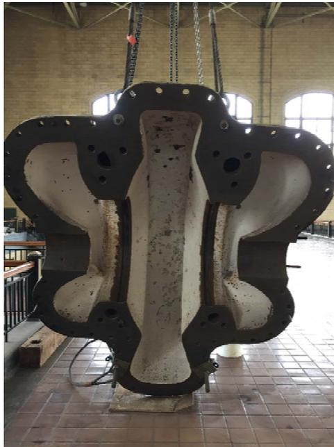
*View of Existing High Lift Pump Impeller Removed for Repairs*
