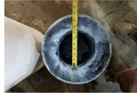
Complex B Sludge Lines clogged due to Struvite
