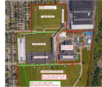
Fire protection loop schematic
