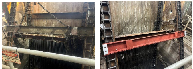
Left: Old chain and rake, right: Replaced chain and rake
