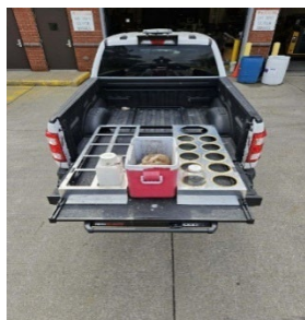
The truck bed slide-out with the fabricated sample holders installed on a laboratory truck
