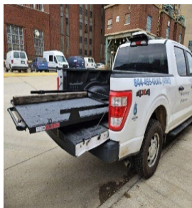
The truck bed slide-out with the fabricated sample holders installed on a laboratory truck
