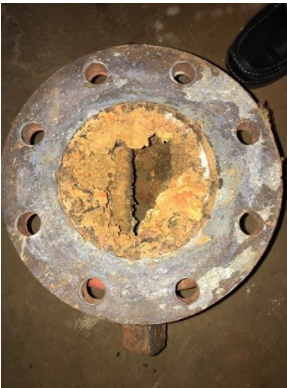
The photo shows the condition of the heating system hot water piping buildup which necessitates the complete replacement of the hot water radiant system in the filter building and other areas of the LH WTP.
