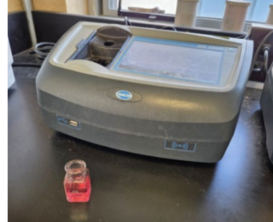
DR3900 with a sample ready to be tested
