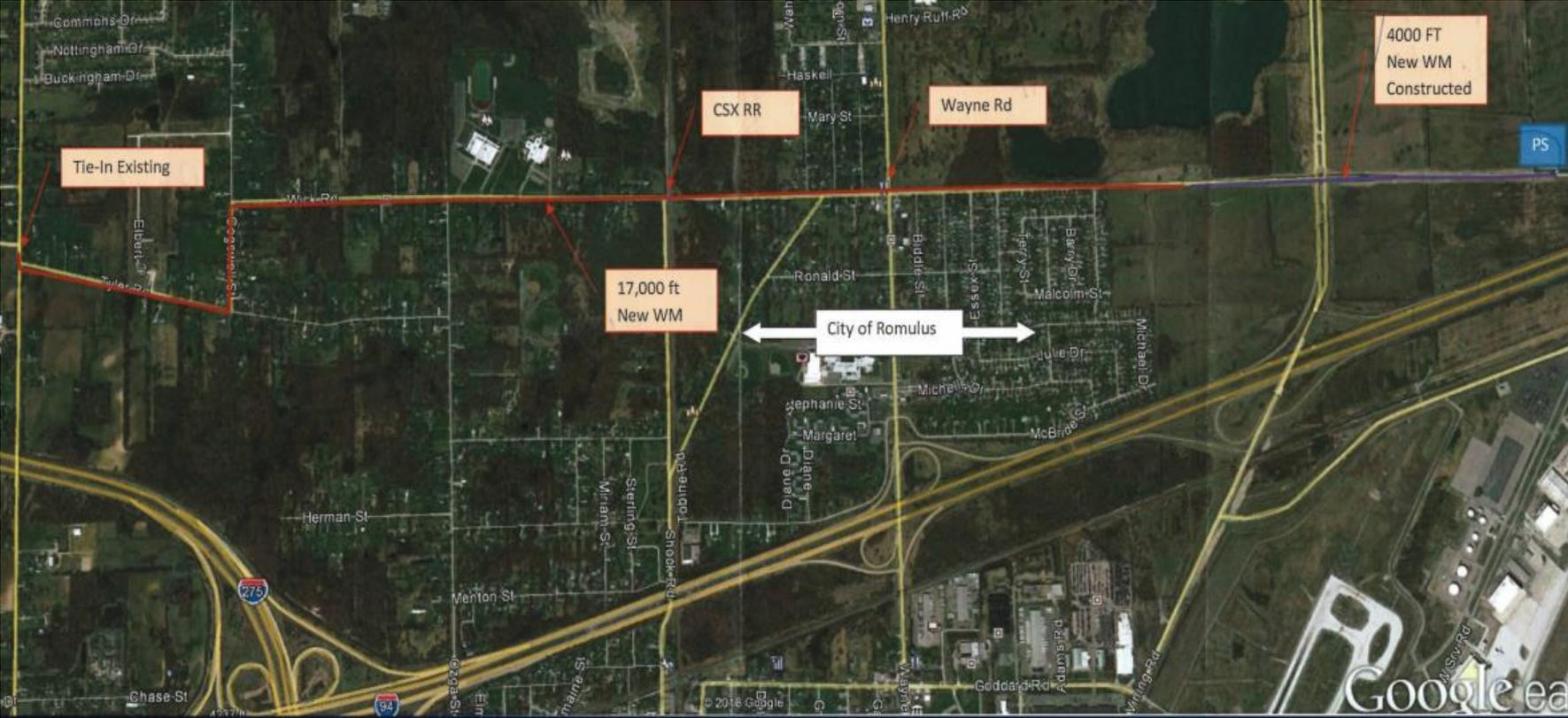
\* Previous 48-inch transmission main was installed in 2013 under MOU-4848, which included roughly 4,000LF of 48-inch main installed to the West of Wick Road Pump Station
