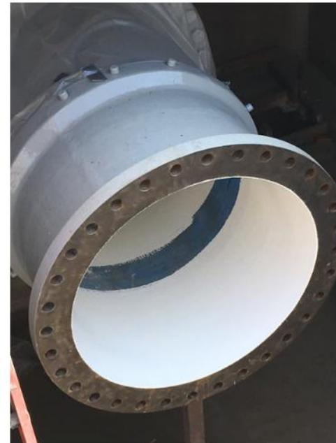
*Photo 6: First coat of paint applied to VM-3 by Dycon at the NEWTP.*
