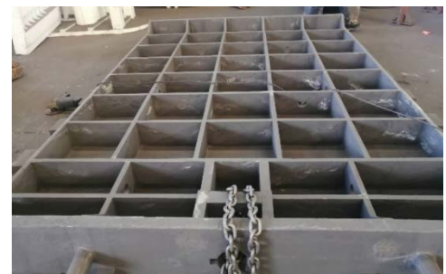
One of eight new isolation gates being manufactured
