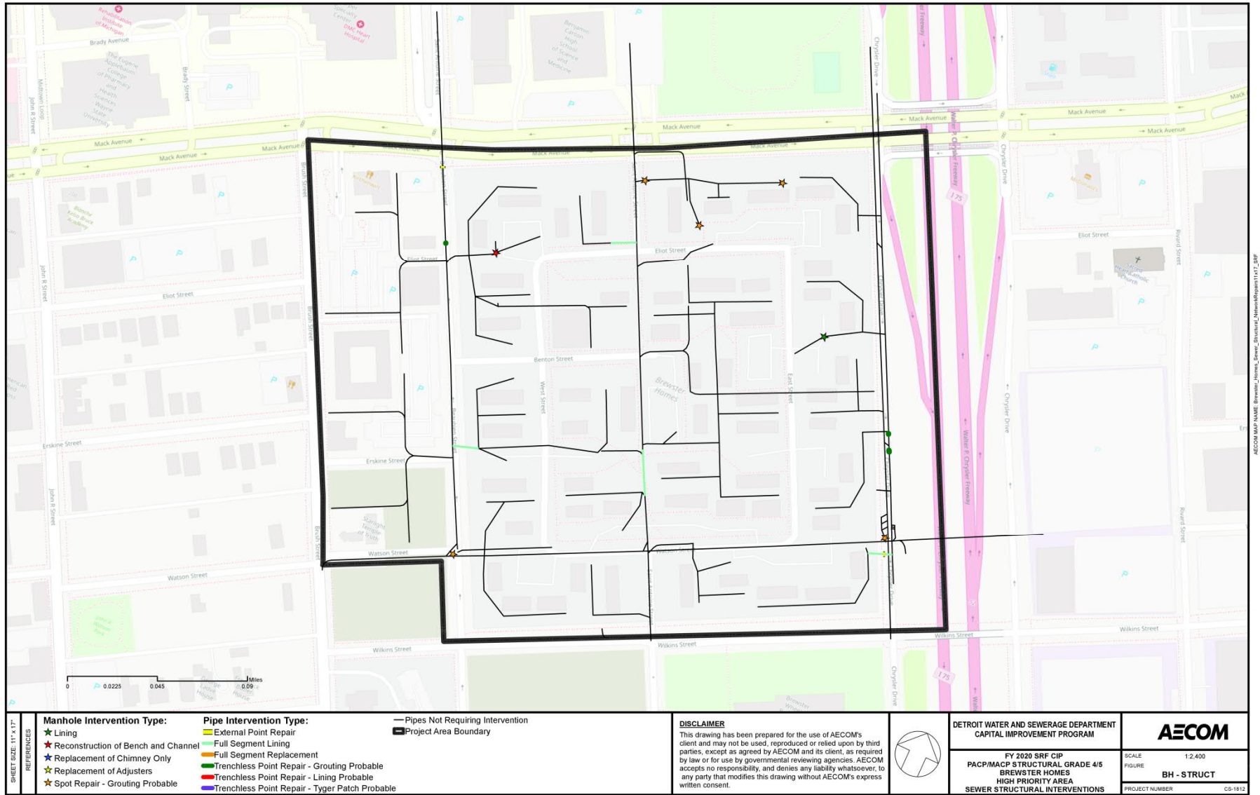
Figure 18 – Brewster Homes Sewer Structural Network Repairs
