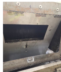
The C belt diverter plate installed at the drop chute.
