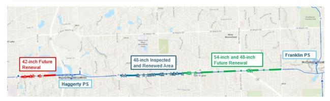
As part of the 7 Mile and Nevada water main project, a 600-foot section of prestressed concrete cylindrical pipe was identified that crossed a portion of I-75. This pipe was taken out of service for the renewal project, which allowed for the opportunistic visual and sounding inspection of the main in late July. The results and recommendation from this inspection are currently being prepared.
