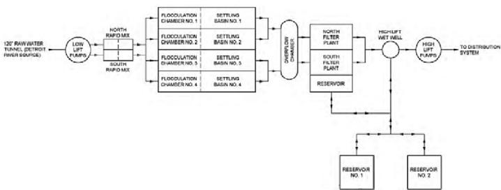
Figure 4. Northeast WTP Process diagram
