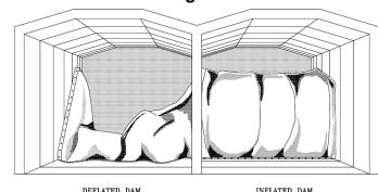
Figure 65. Inflatable dam illustration
