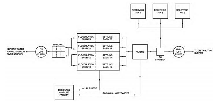
Figure 7. Southwest WTP process diagram
