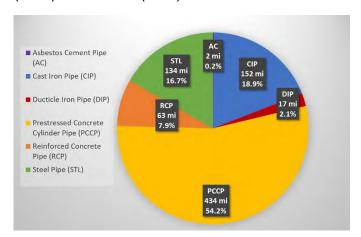
Figure 12. Transmission system inventory by material
