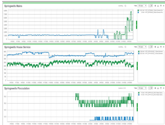
Springwells Metering Data from Power Monitoring Expert (PME) Software
