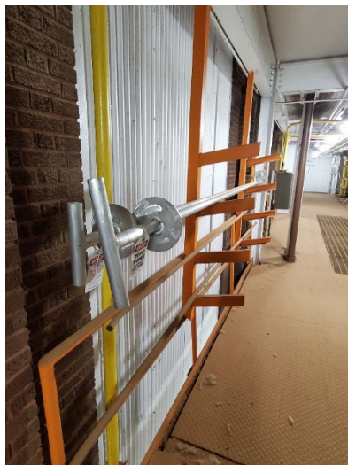
New tools manufactured as a trial program. These tools are significantly lighter than the old steel tools and should be easier to use
