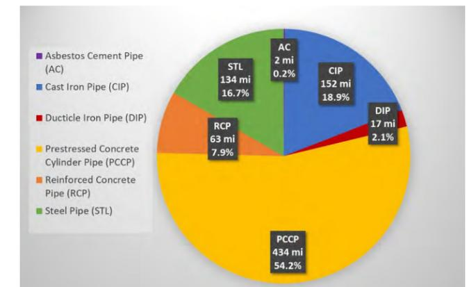
**Figure 12. Transmission system inventory by material**
