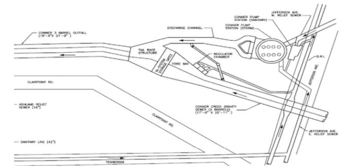
**Figure 56. Schematic of Conner Creek Pump Station**
