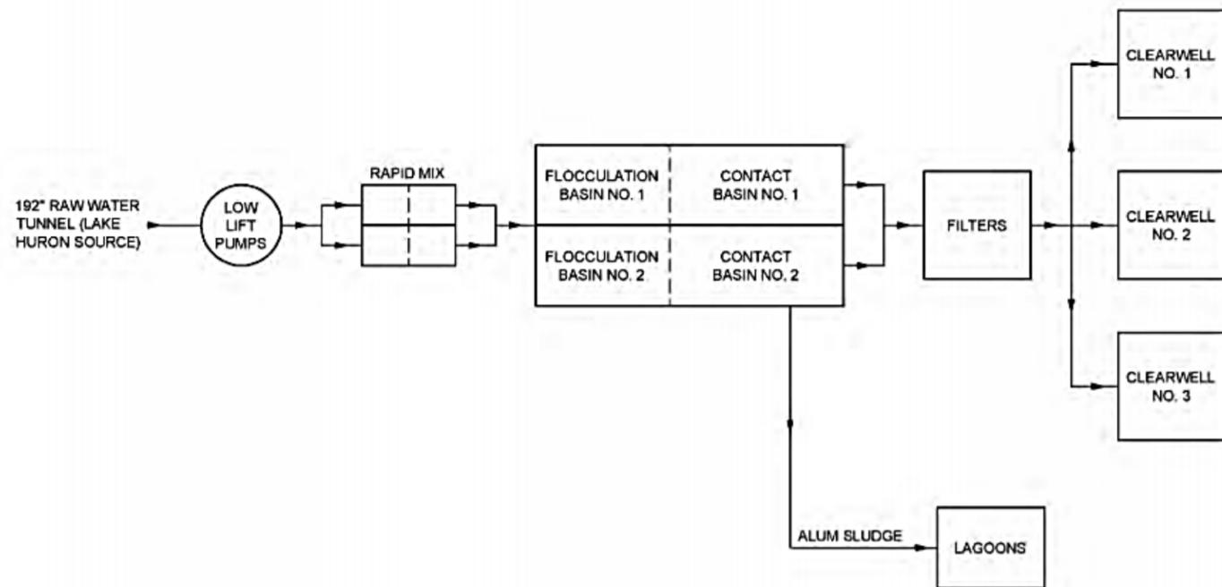
Figure 2. Lake Huron WTP process diagram
