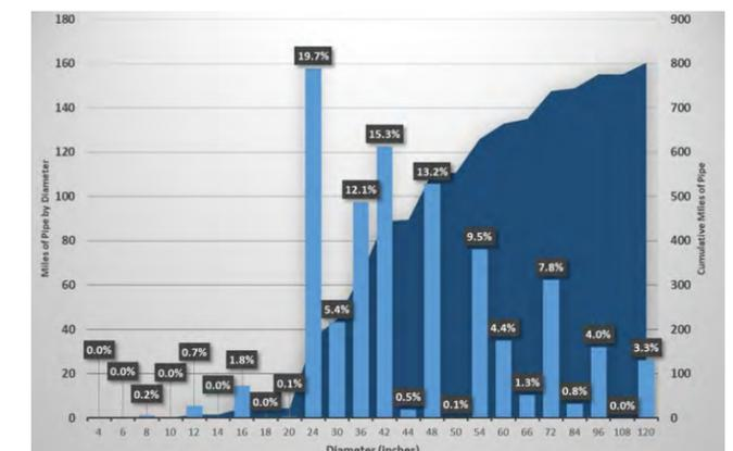
**Figure 13. Transmission system inventory by diameter**
