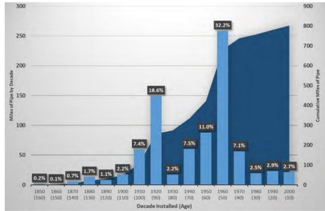
**Figure 14. Transmission system inventory by decade installed / age**
