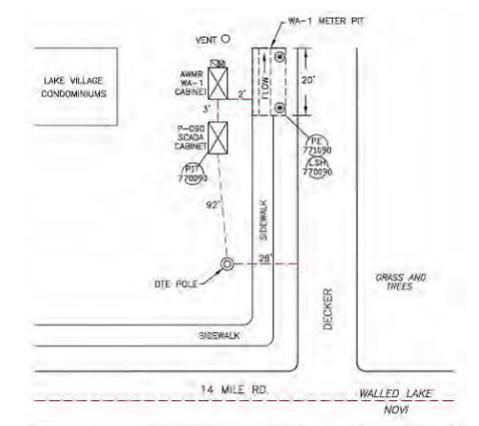
**Figure 17. Pressure Monitoring Site at 14 Mile and Decker**
