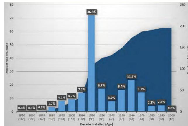
**Figure 50. Collection system inventory by decade installed/age**
