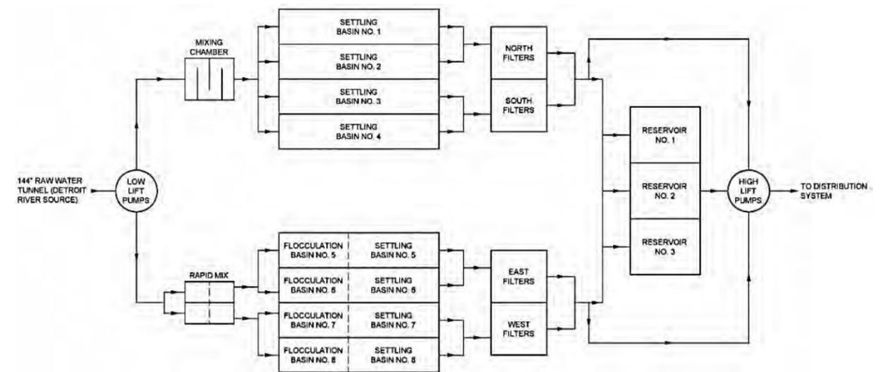
**Figure 9. Springwells WTP process diagram**
