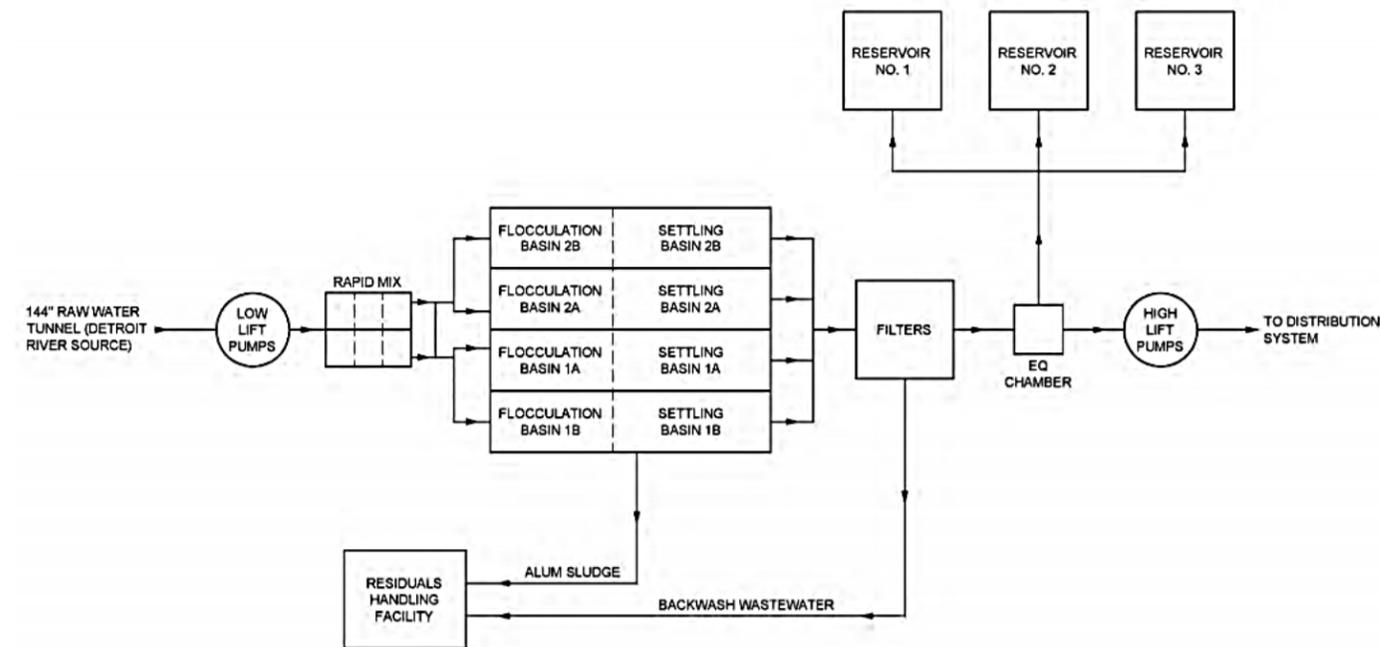
**Figure 7. Southwest WTP process diagram**
